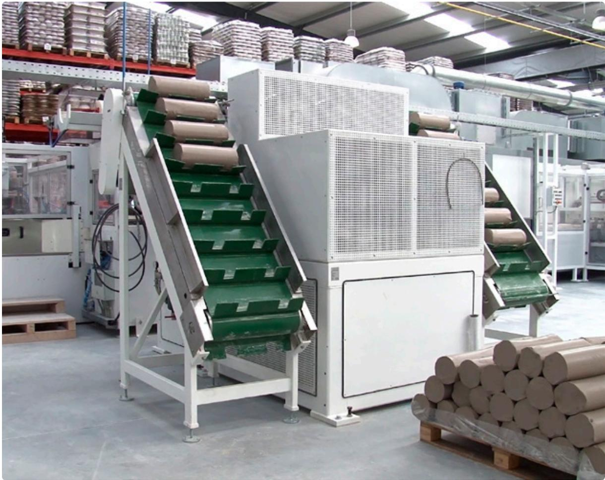
The SACMI-SAMA range comes complete with an extruder that makes the pugs used in the shaping process. Two options are available: extruder integrated in the machine to rework already-extruded material or a stand-alone machine for the extrusion of filtered cakes.
