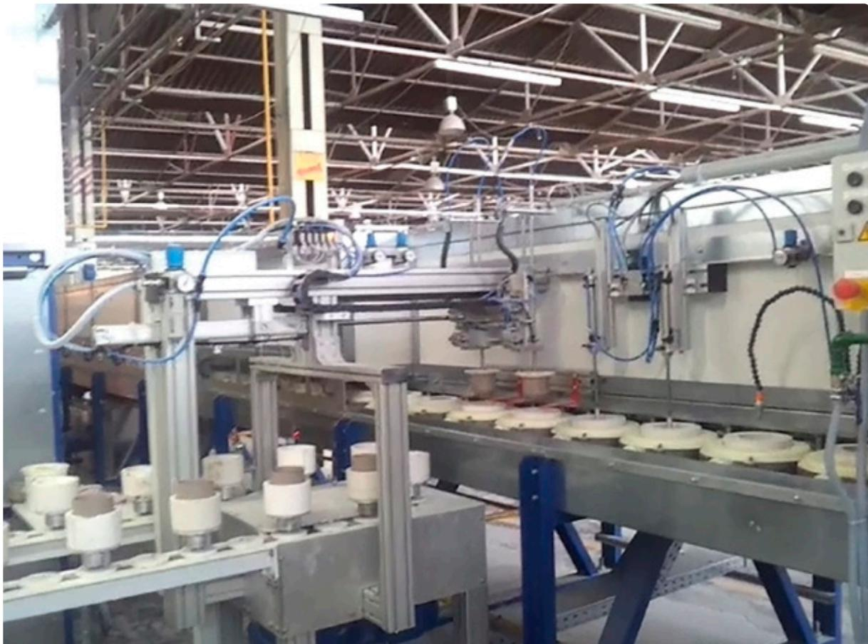
The roller heads can perform a horizontal retraction movement during shaping.
